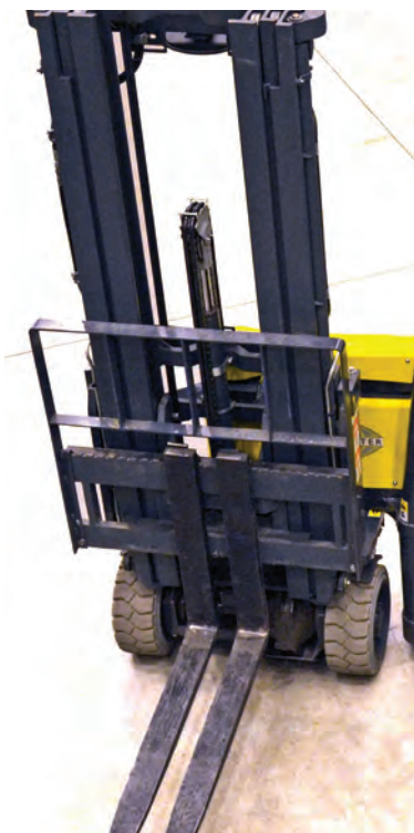
High rack lifts place higher demands on floor joints due to their smaller harder wheels and increased point loads.
